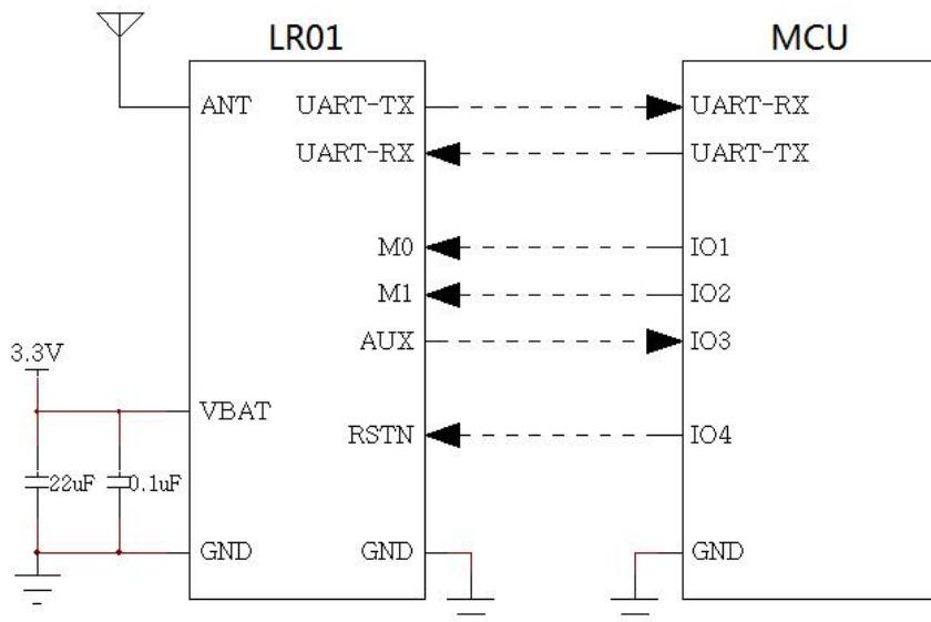
Figure 2 Module minimum system diagram
