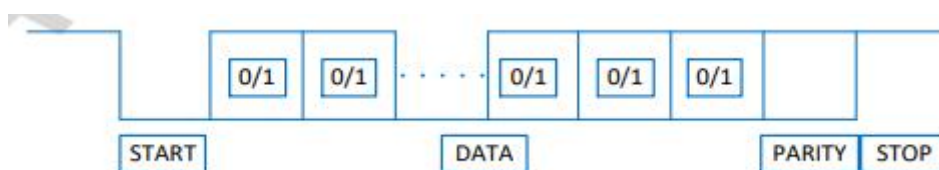
Figure 12 LPUART data transmission format
